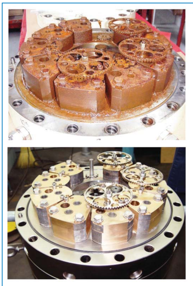
Figure C Corroded flow divider, top. Upgraded flow divider, bottom.
